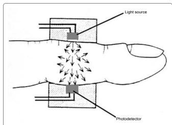
Figure 1: Photoplethysmography. (Source:http://sashpsg.blogspot.com/2015/02/photoplethysmography.html)
