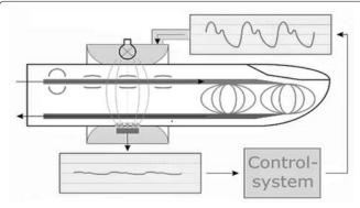
Figure 2: Volume clamping. (Source: https://en.wikipedia.org/wiki/Continuous\_noninvasive\_arterial\_pressure)
