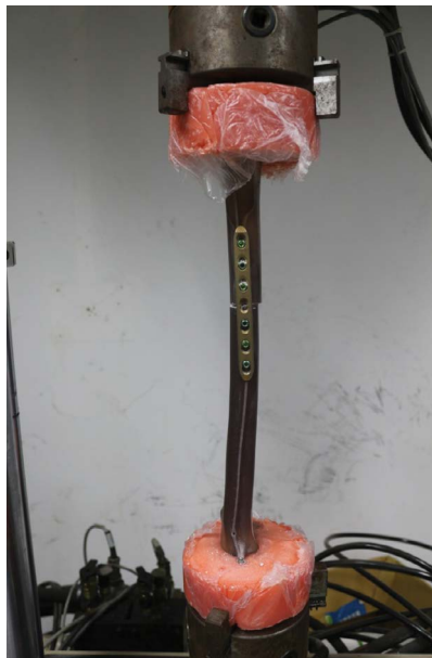
Figure 6: The torsion test on an MTS 858
