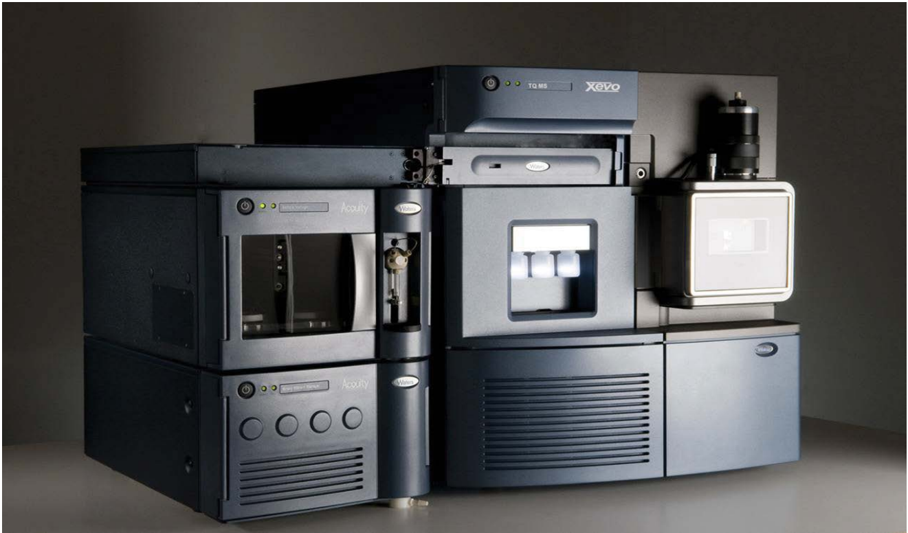
Figure 1: UPLC Acquity Ultra Performance LC XevoTQ MS. Equipment used for measuring antibiotic concentrations by mass spectrometry.
