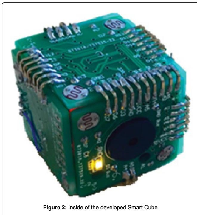
Figure 2: Inside of the developed Smart Cube.
