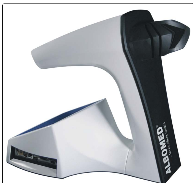
Figure 1: Picture of the device, PupilX. The participant needs to look into the black light-tight rubber eyecups. The investigator could monitor all data at the screen sinistral at this picture. [www.albomed.de]
