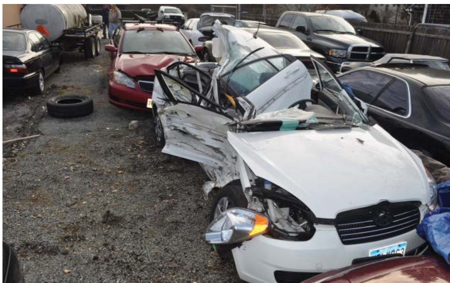
Figure 6: View of passenger vehicle demonstrating at least 12 inches of side impact movement.
